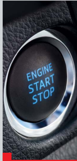
Push Start To start the engine, simply push down on the brake pedal then press the start button while the key is in range.
