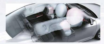
SRS (Supplemental Restraint System) airbags for the driver, front passenger seat, sides and curtain shields help reduce the collision energy imparted to occupants in the event of a collision.
