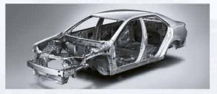
Camry's impact absorbing body is designed to disperse and absorb collision energy to control excessive cabin deformation and ensure passenger safety.
