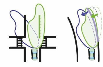
Camry's AFS (Adaptive Front Lighting System) technology changes the headlamp beam direction in response to steering operations, increasing visibility at intersections and turnings.
